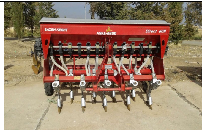
Fig. 1 : No till seeder with row cleaner modification front view
